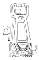
4. Slide the power cord hook into position of unit right.
