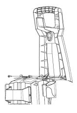
2. Installing the accessory board into position with two screws.
