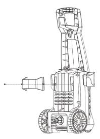
3. Slide the trigger gun holder into position of unit left.
