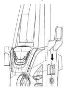
5. Installing the two wheels.
