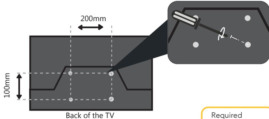
The TV comes with holes on the back panel for use with wall-mounting brackets (bracket not included).
