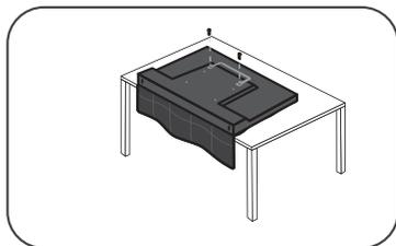
1. Remove the metal handheld bracket from the box and align the handle with the holes top two hole on the back of the TV.
