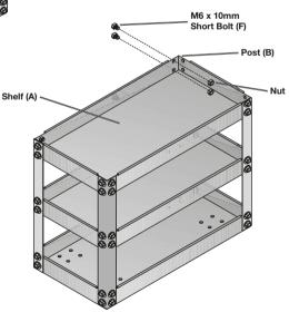
Attach the last Shelf (A) to the inside top of the Posts (B) using twelve Short Bolt and Nut Sets (F) - 1x M6 x 10mm Short Bolt and 1x M6 Nut per set. (Four holes on one end of this top Shelf (A) are reserved for attaching the Tubular Steel Handle (E) in the next step.)
